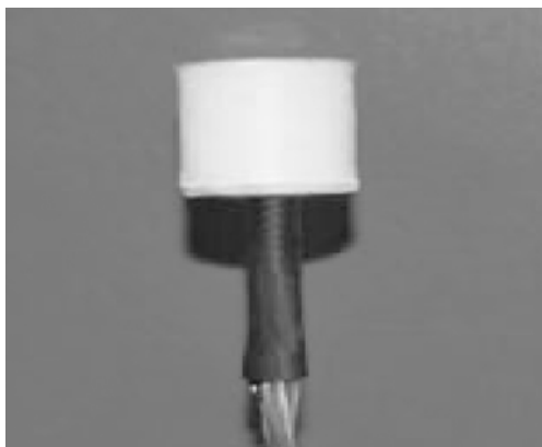
Fig. 2 Photograph of the heat transfer coefficient sensor
